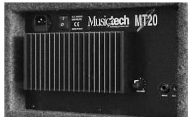
Details of MT 20 rear mounted control panel
